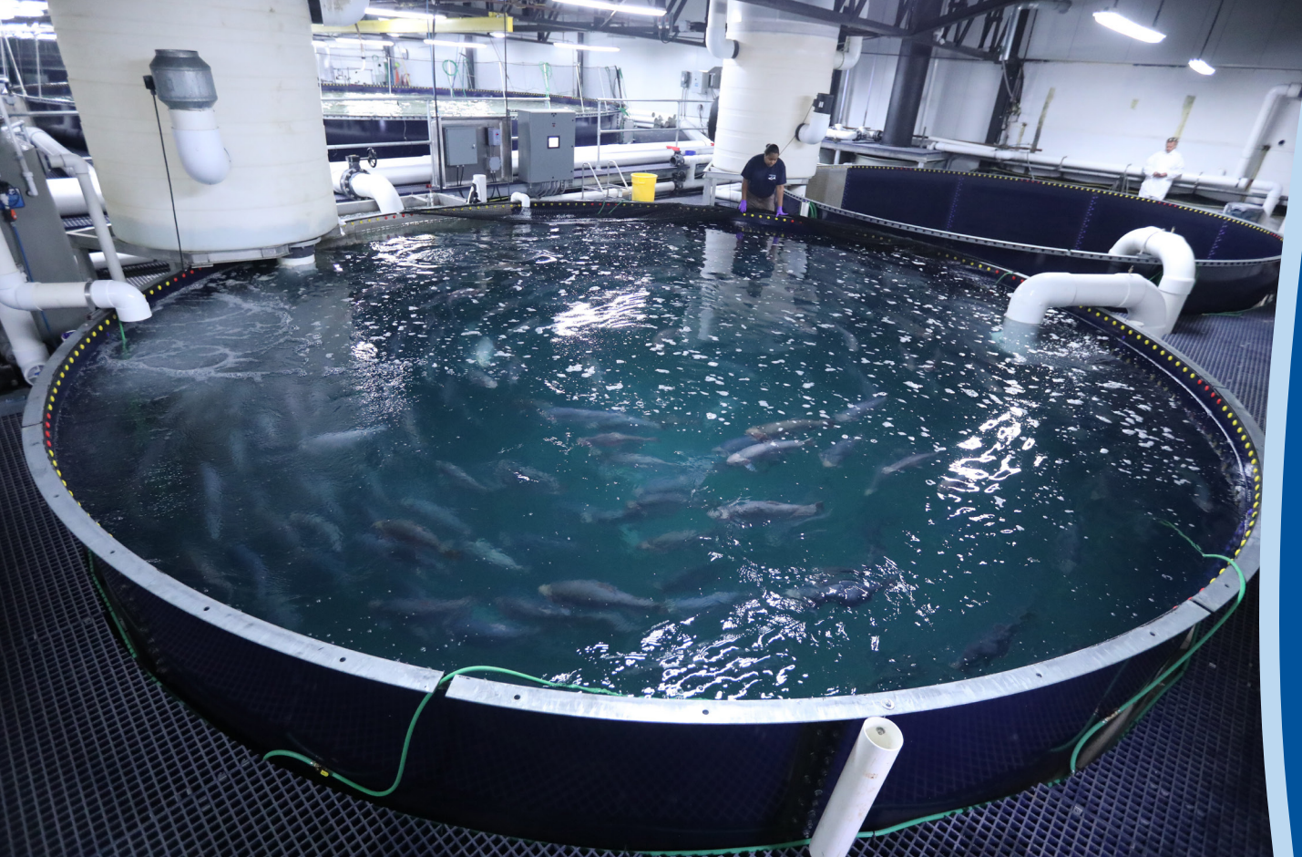
Commercial scale recirculating system culturing steelhead trout. Image credit: John Ng/Hudson Valley Fisheries
