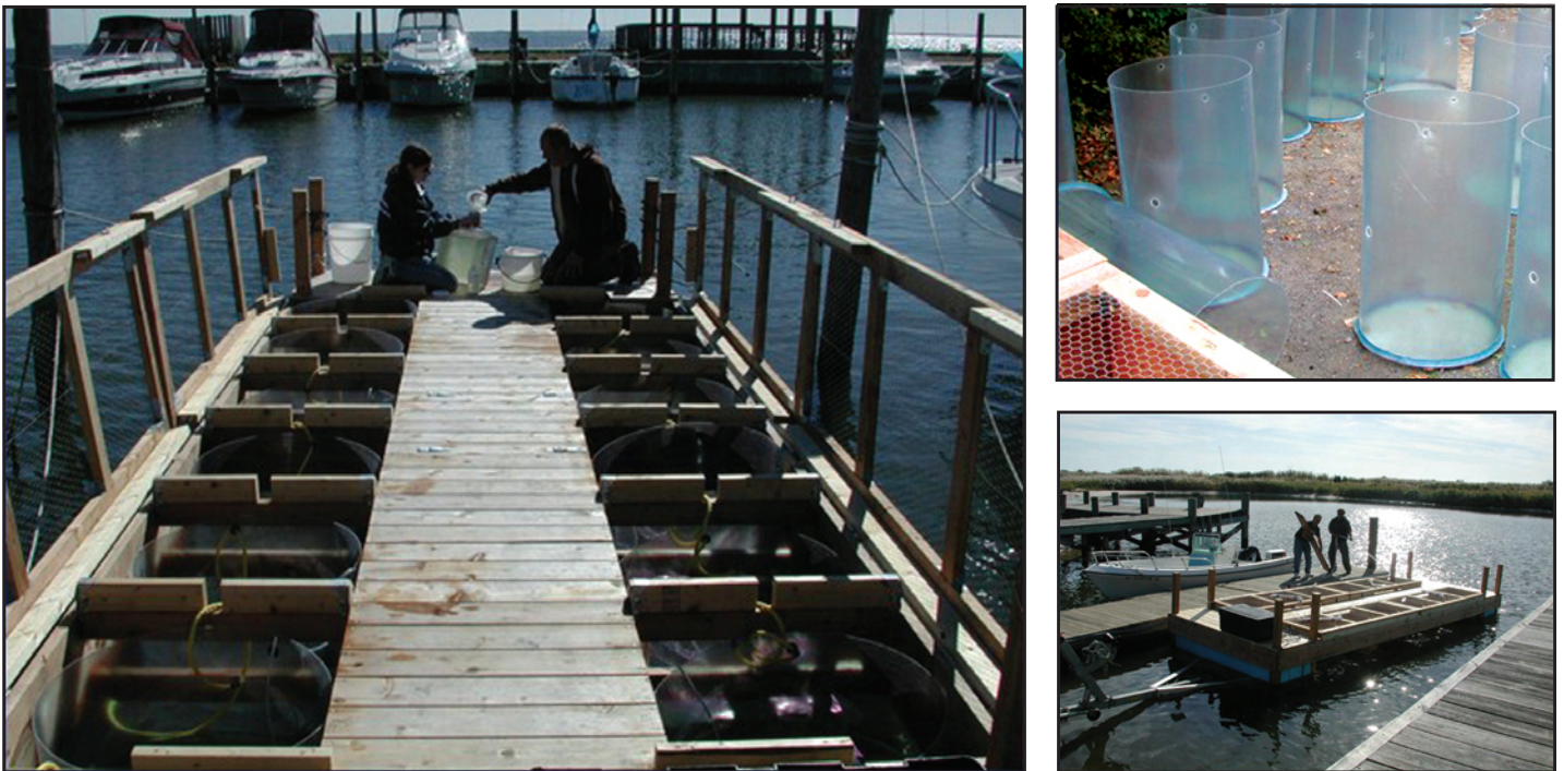
Figure 19. View of moored platforms deployed in the field during the spring and summer of 2002 (Streck 2003 and Cerrato et al. unpublished). The 2.4 x 6.7 m (8' x 22') platform had a center walkway and held 12 fiberglass cylindrical tanks containing 400 L seawater, suspended from each side (also shown in the inset), covered with screened doors.
